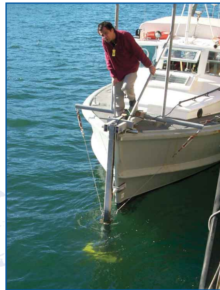
Multibeam sonar head mounted on boat Source: DSTO
