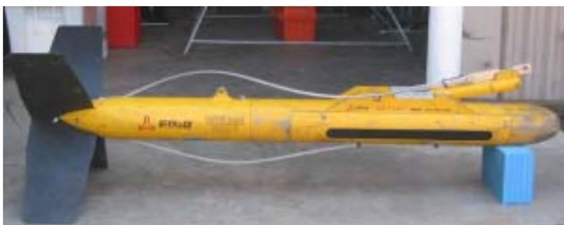
**Figure 2.1 Edgetech 272 sidescan sonar ‘fish’ used in CBMP survey**
