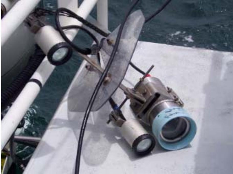
**Figure 2.4 Towed video camera with lights**
