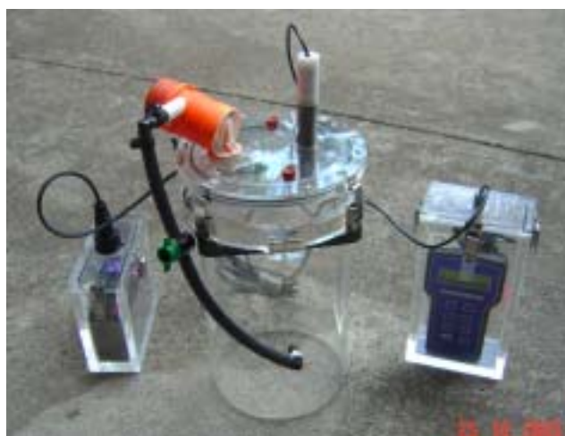
Figure 3: Benthic chamber as used in benthic metabolism and benthic flux measurements. The dispersion attachment for mixing is not shown in this picture.
