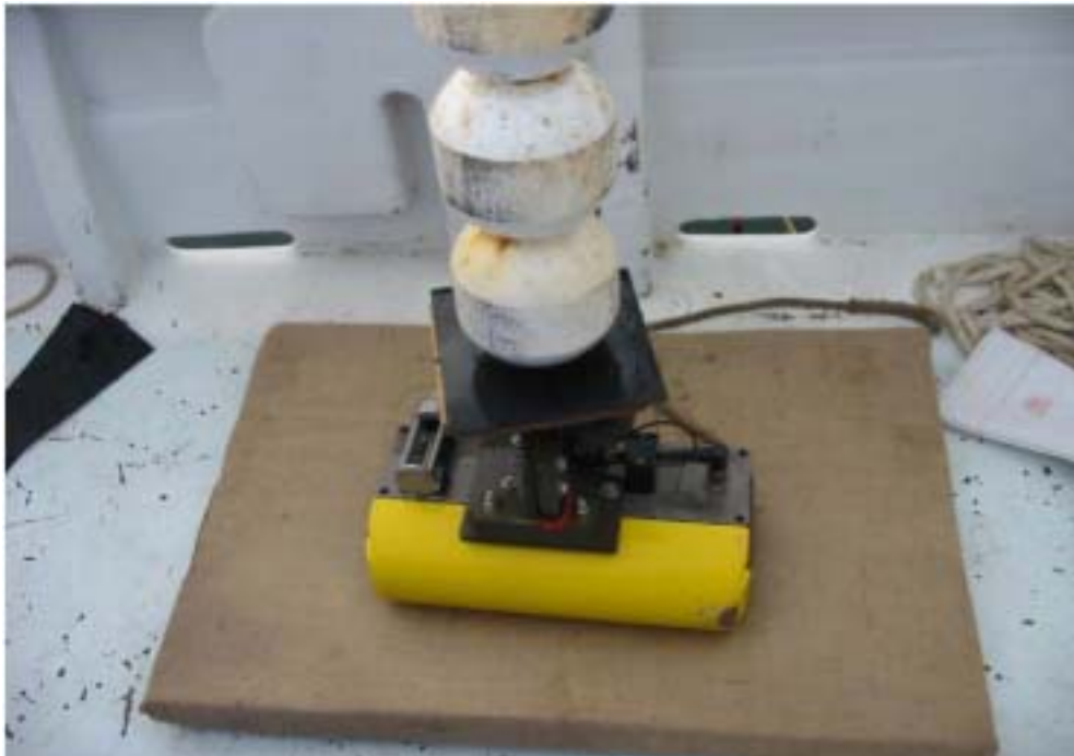
Figure 17. Reson 8125 transducer head (forward end) mounted for fitting in a large-diameter sonar well of a pilchard fishing vessel
