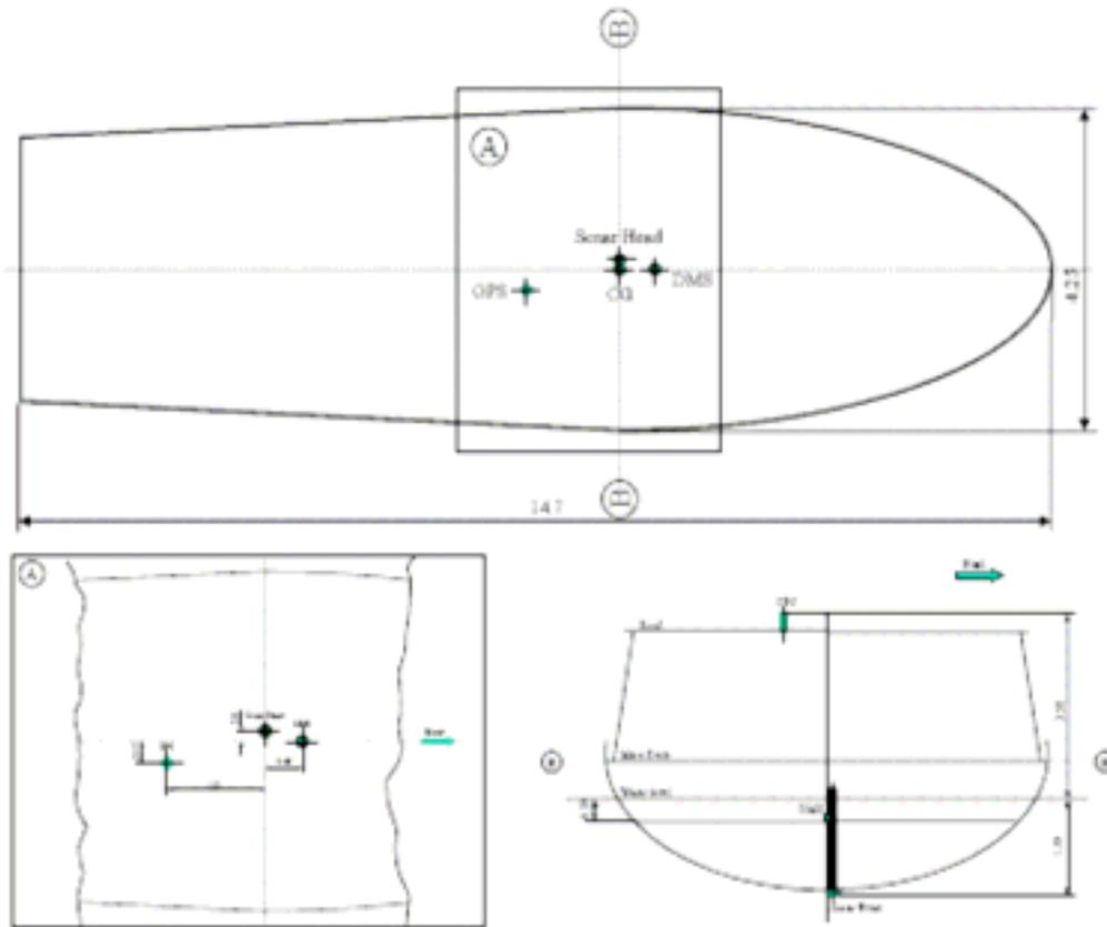
**Figure 22. Layout of the various sensors on a vessel for a multibeam survey**
