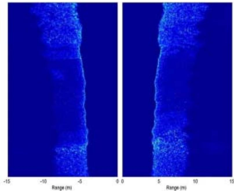
**Figure 12. Example of sidescan output (synthesised from multibeam data) showing the water column aside nadir (uniform blue adjacent centre of plot), and seagrass (the textured portion of sidescan output at top and bottom of plot) with a sand patch in between (clear section through plot centre)**
