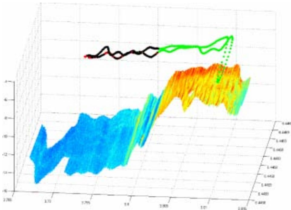
Figure 16. Comparison of results derived from the multibeam (as shown in Figure 15) and the single beam systems over a sand and seagrass bottom
