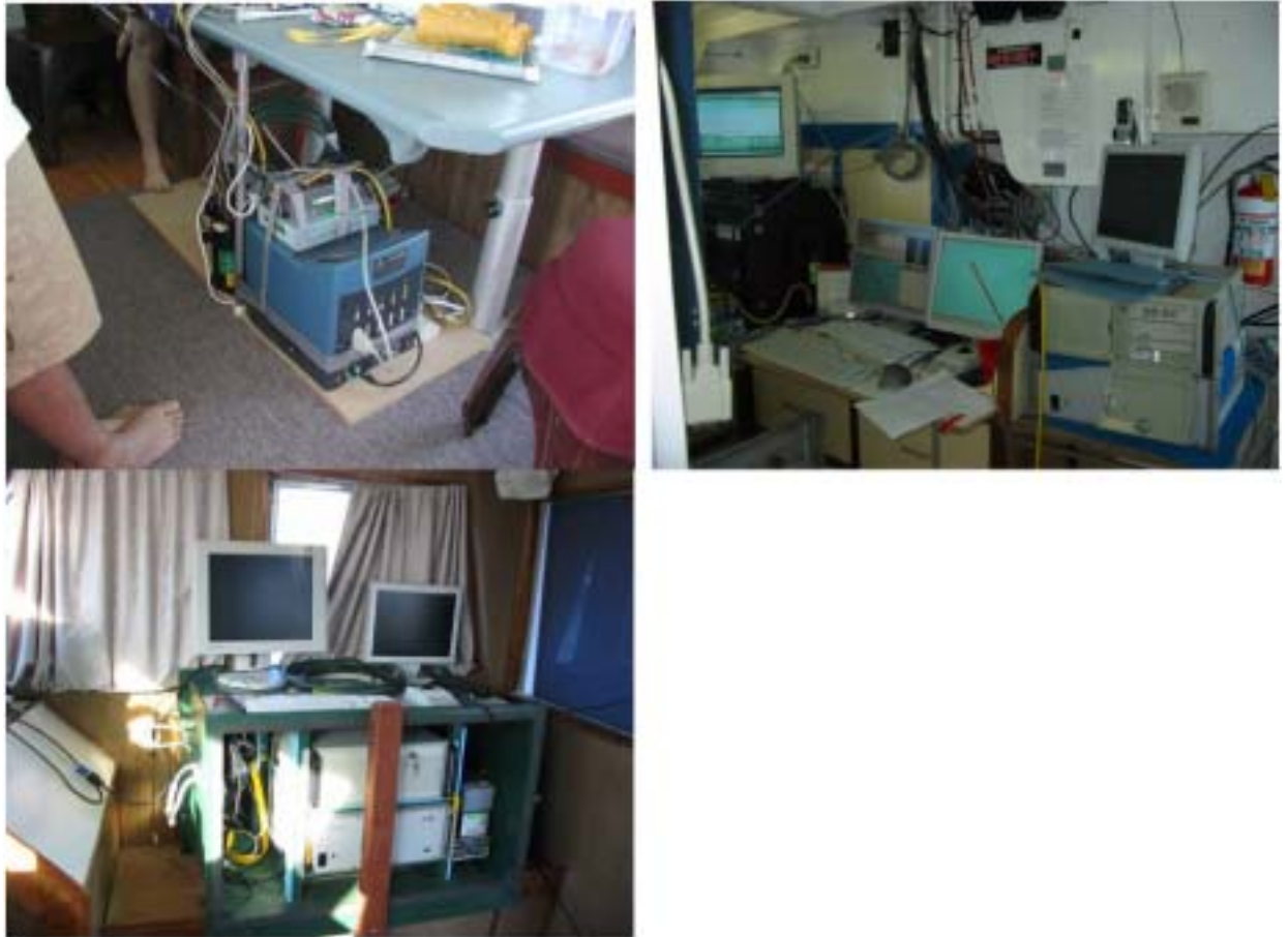
Figure 21. Images of a RESON SeaBat 8125 sonar system
