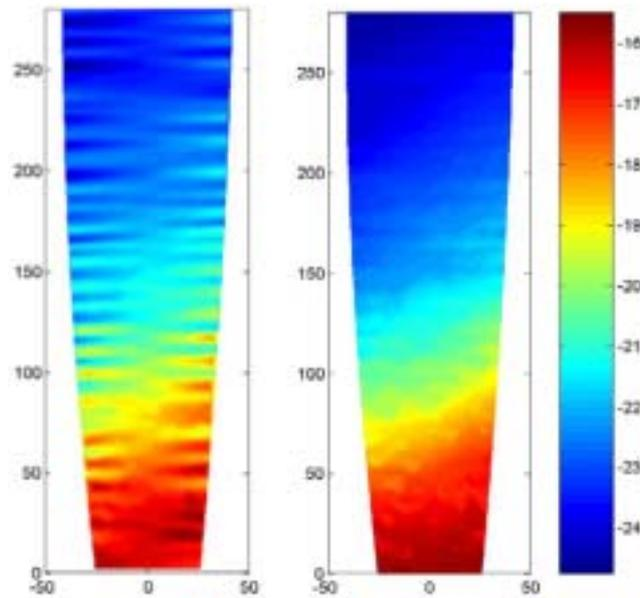
**Figure 5. Bathymetry images before (left panel) and after (right panel) compensation for ship's motion**
