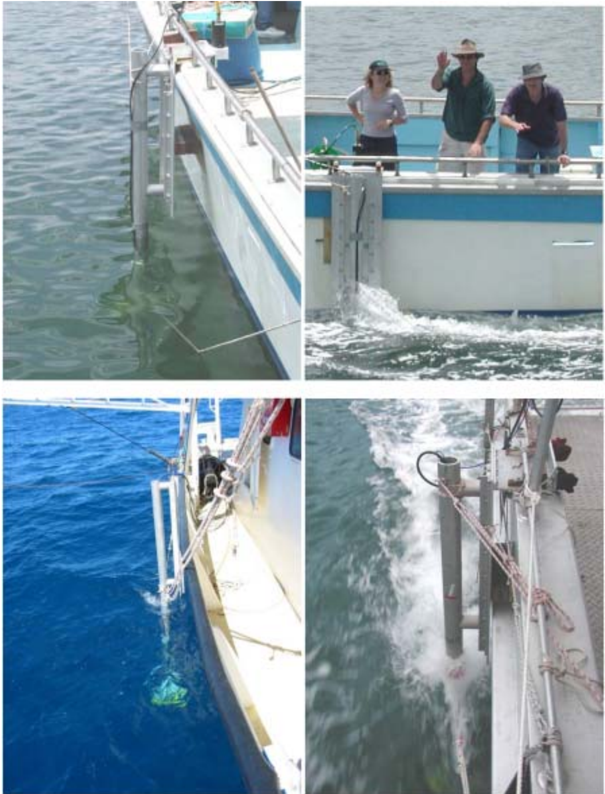
Figure 19. Images of a Reson 8125 pole mounted off the gunwale of three vessels
