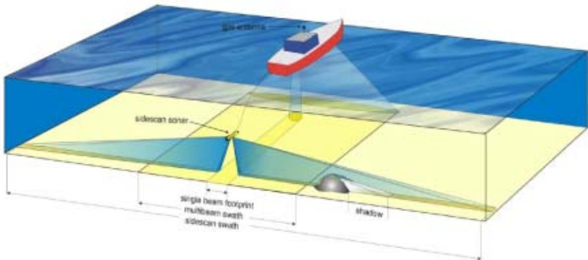
**Figure 1. Comparison of coverage between acoustic mapping technologies**
