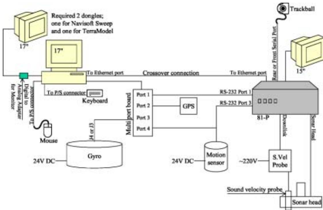
**Figure 20. Schematic diagram of setup required for multibeam hardware aboard vessel**
