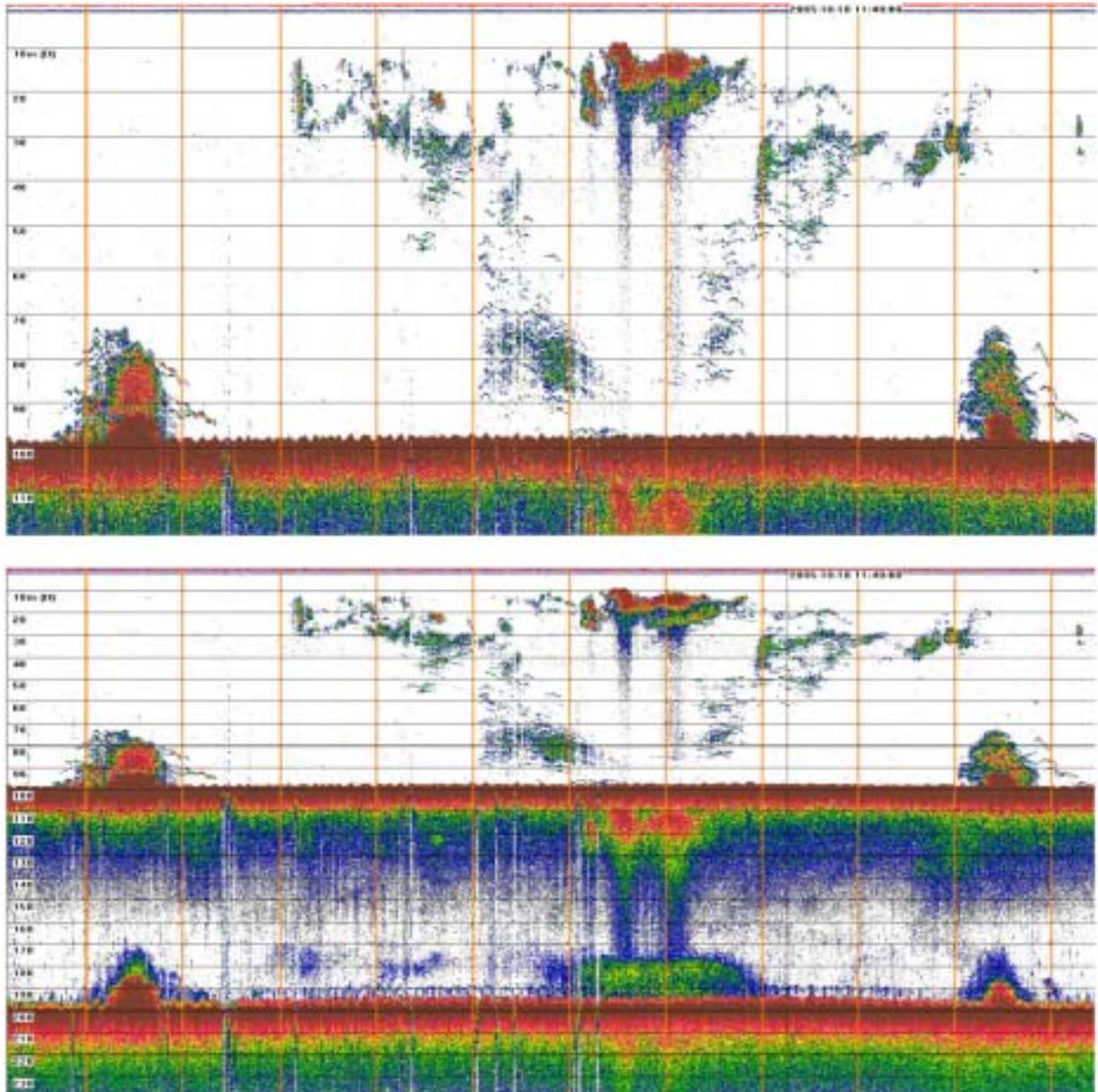
**Figure 8. Example of single-beam sonar output showing (top) strong water column scatterers and (bottom) the same time-frame showing the strong second echo from a hard limestone bottom with a thin veneer of overlying sand**
