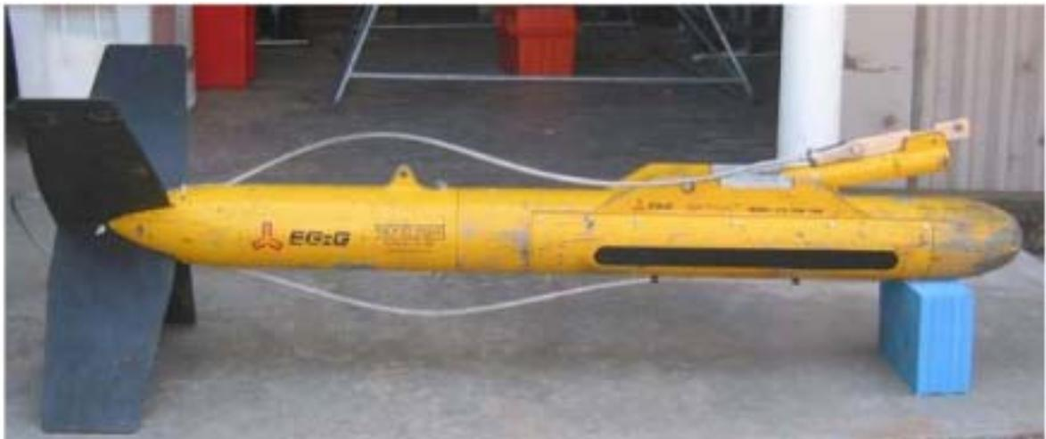
**Figure 3. Typical sidescan sonar fish**
