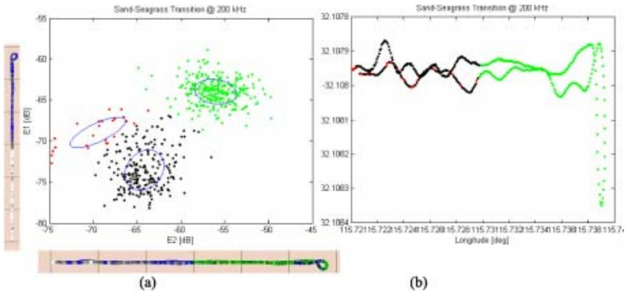
Figure 10. Scatterplot of E1 vs. E2 after cluster analysis (a) and seabed habitat classes along the track (b)
