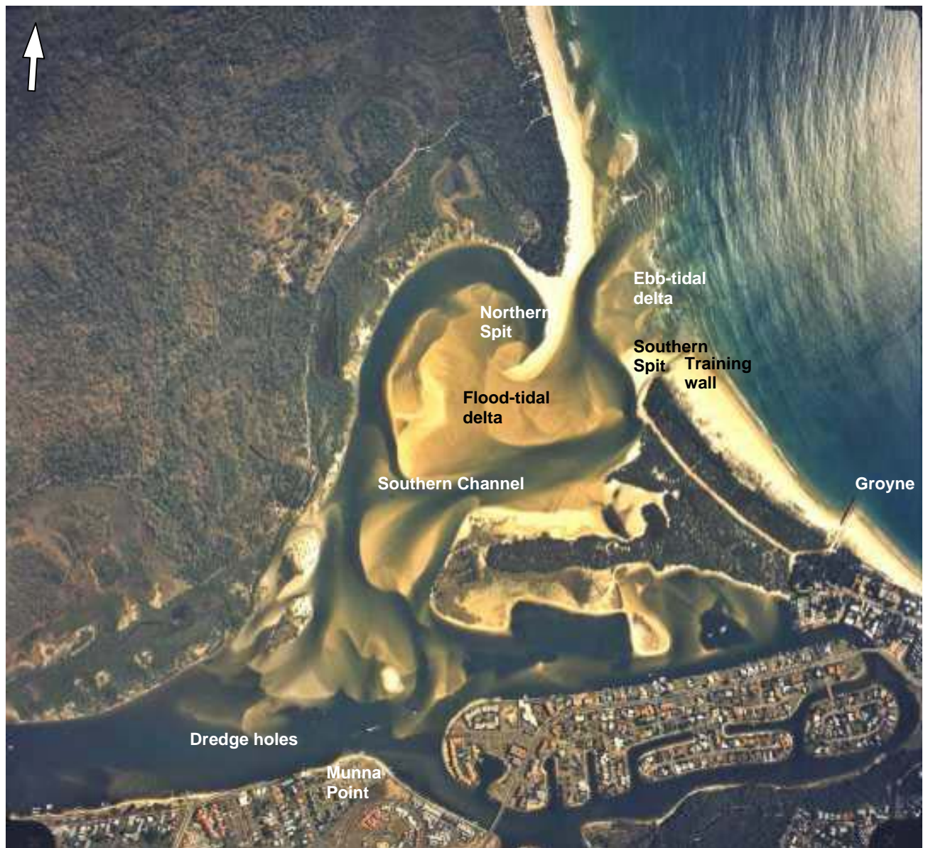
Figure 26. Noosa beach and estuary system, 28 August 1986 (Source: Beach Protection Aerial Photography, 1986)
