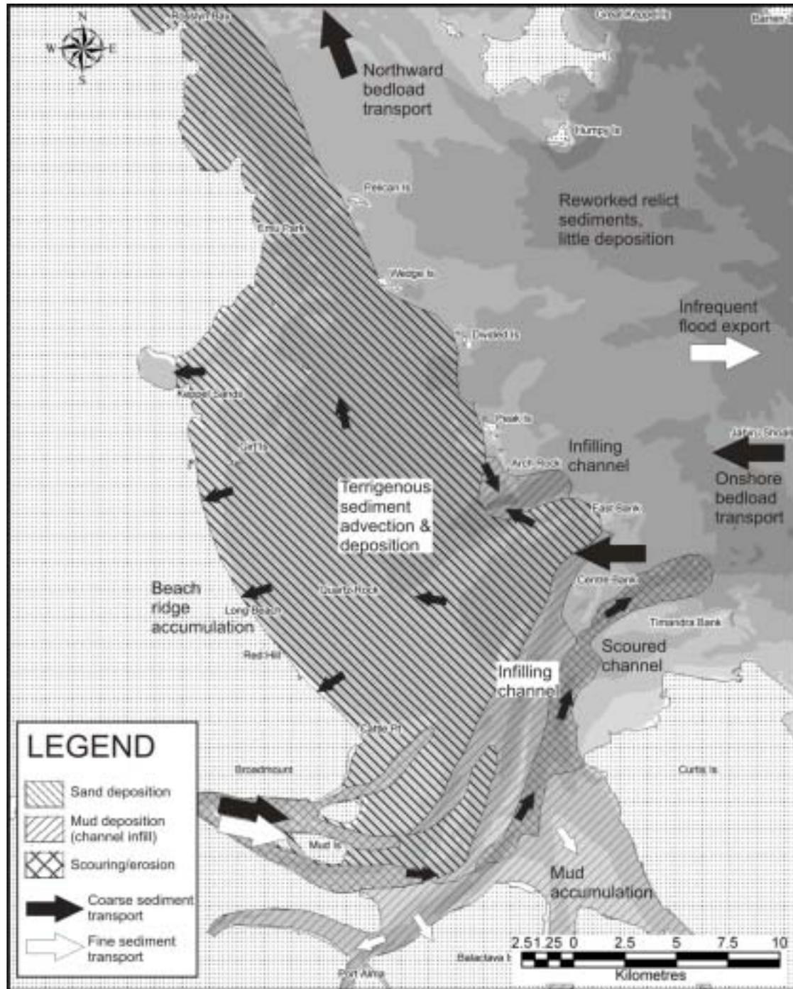
Figure 2: Map of sediment transport, accumulation and erosion in Keppel Bay.
