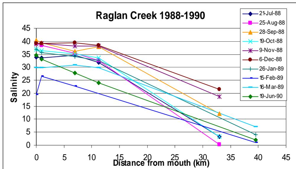
Figure 11. Longitudinal conductivity in Raglan Creek, 1988-1990 (Data: EPA)
