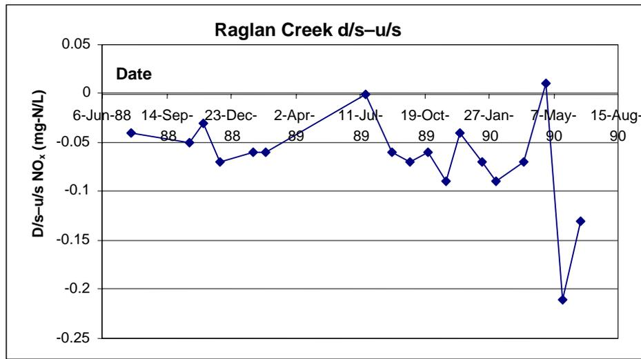
**Figure 13. Concentration difference for NO<sub>x</sub> between downstream (d/s) and upstream (u/s) stations in Raglan Creek, 1988–1990 (Data: EPA)**
