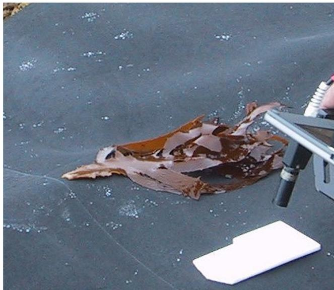
**Figure 4** Example of measuring panel radiance (from a Teflon reference panel) with an ASD field spectrometer prior to reflectance sampling of *Ecklonia* over black neoprene (image source: Dekker et al, 2003)
