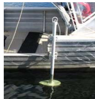
Pole-mounted single-beam transducer on a small vessel
