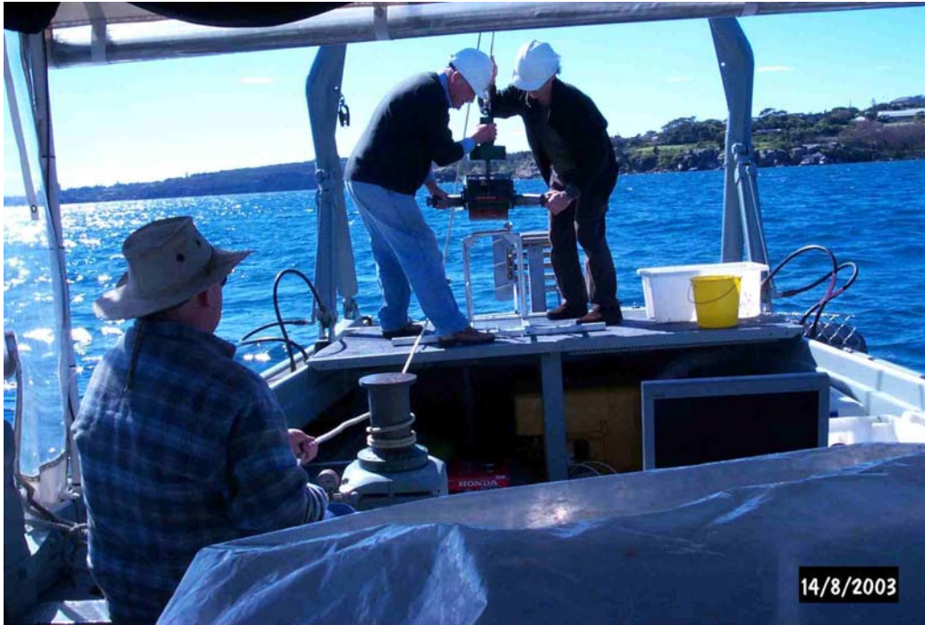
Figure 3a - Deployment of the Smith-Mackintyre Grab for sand and muddy sand sediments.
