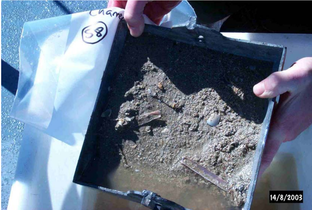
Figure 4a - Muddy sand sediment collected using the Smith-Mackintyre Grab Sampler (Site 58).
