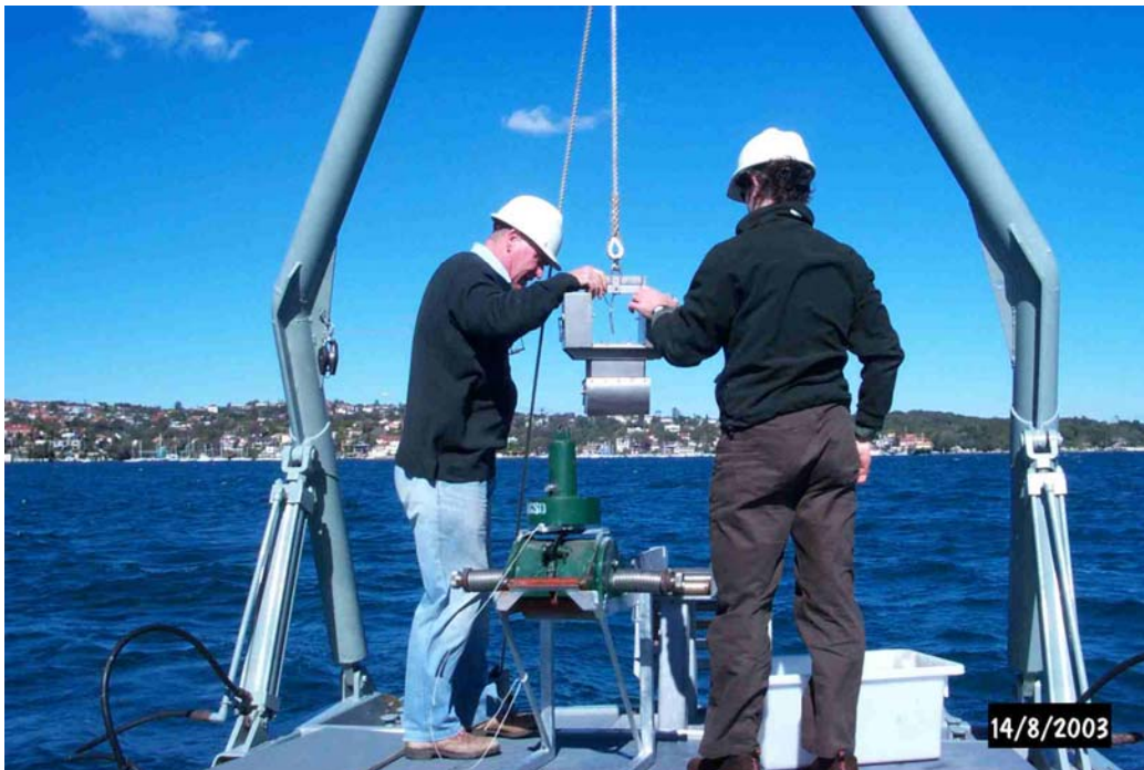
Figure 3b - Deployment of the Box Corer for undisturbed mud sediments.
