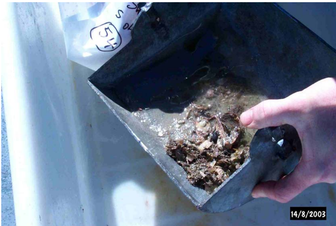
Figure 4a - Muddy sand sediment collected using the Smith-Mackintyre Grab Sampler (Site 58).
