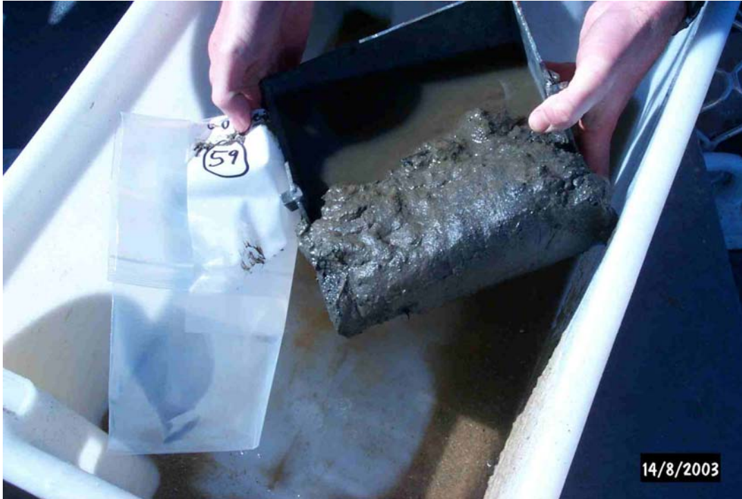
Figure 4c - Muddy sediment collected using the Smith-Mackintyre Grab Sampler (Site 59). Most mud sites were targeted using the Box Corer.
