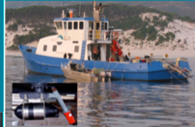
Above: Multibeam platform, FRV Challenger. Inset 8101 multibeam and USBL video position transponder
