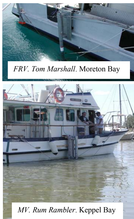
Figure 2. Photographs showing the sonar head side-mounted on the boat used in the survey.
