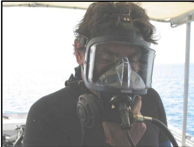
Figure 4. Kim Nardi from the Department of Fisheries, Western Australia wears a full-face mask in which he makes voice recordings of all fish seen within the transects boundaries. The voice recordings are directly overlaid onto the video images captured by the left camera (Figure 2).
