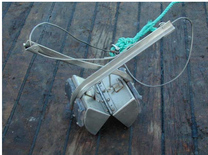
Figure 6: Small (0.5 litre) stainless steel Van Veen grab.
