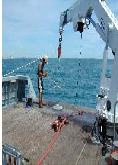
Figure 7: Larger Van Veen grab loaded and ready for deployment.
