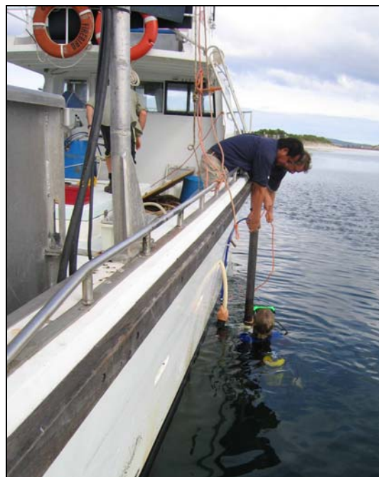
Figure 4: Installing the Reson 8125 sonar head on the Jumbo . The mounting pole was inserted into a moon pool within the hull of the boat.
