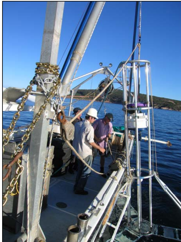
Figure 7: Deploying the vibracorer over the side of the Jumbo using the very effective two winch setup.
