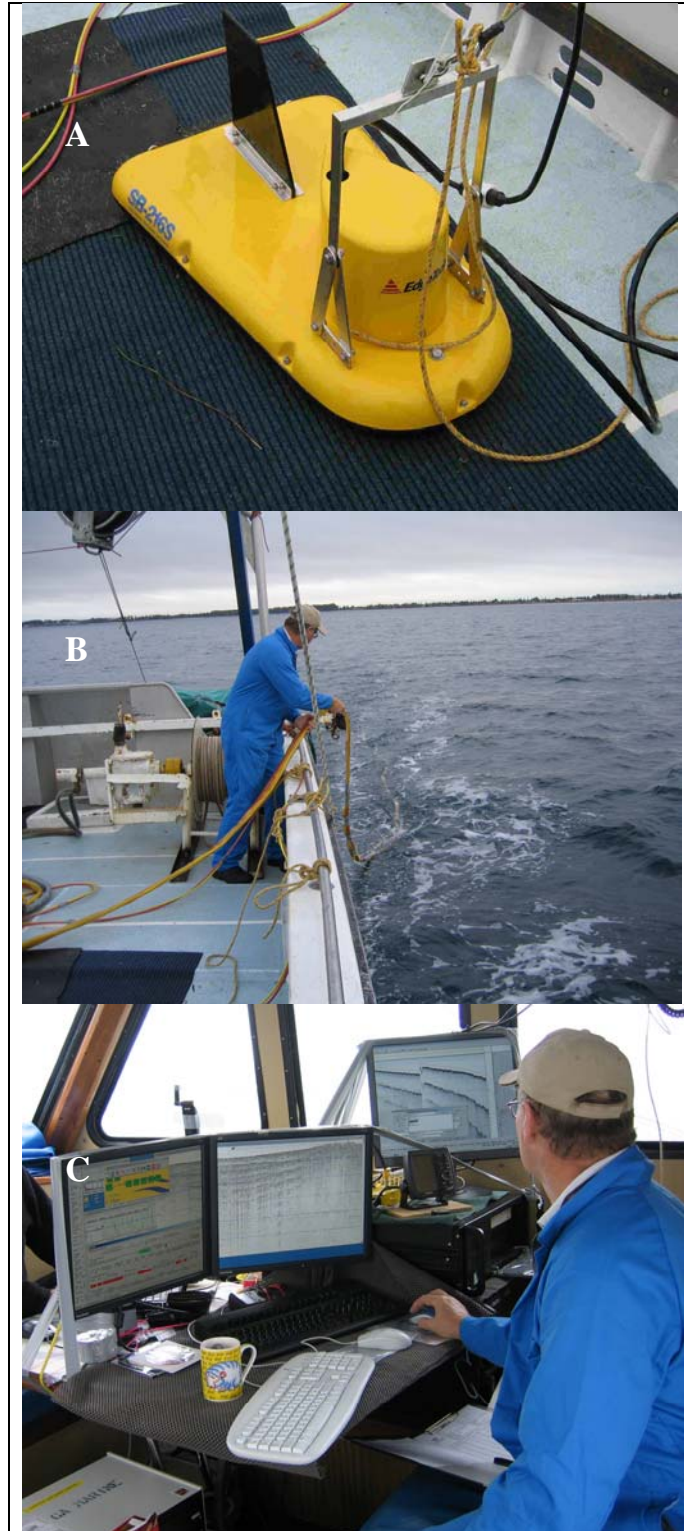
Figure 3: A) Tow fish unit of the Edgetech SB-216S ‘Chirper’ sub-bottom profiling system. B) Deploying the high voltage signal cable of the ‘Sparker’ system. C) Screen displays and integrated data acquisition unit for the three sub-bottom profiling systems, set up in the wheel house of the Jumbo .
