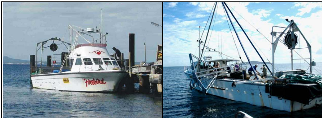
Figure 2: The Firebird (14 m) and Jumbo (17.2 m) vessels used in the survey. The Jumbo has the vibracorer set ready for deployment.
