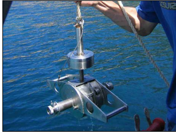
Figure 8: The mini-Shipeck grab sampler used in the survey to collect samples of surface sediment.
