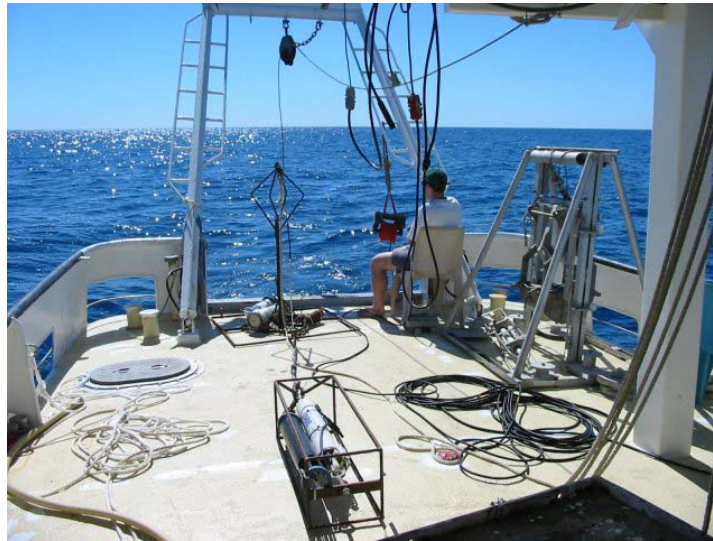
Figure 5. Iain Parnum enjoying the scene while holding the umbilical of the UWA underwater video camera. Also seen in the photograph are the CTD/SVP and the tide gauge deployed in Bowling Green Bay.
