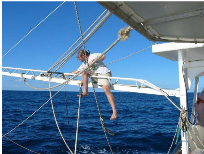
Figure 6. Thomas Stieglitz measuring the offset of the head of DATASONIC CHIRP-660 sub-bottom profiler relative to the GPS antenna.
