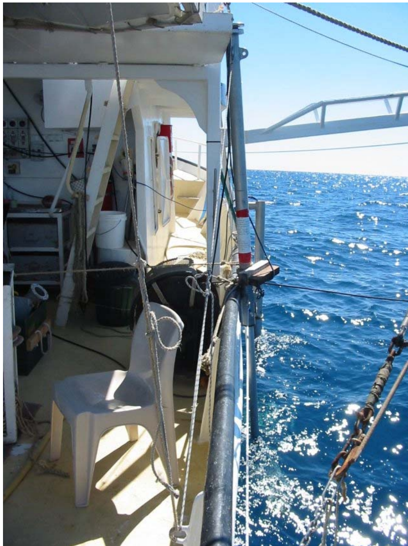
Figure 2. The mounting poles used to mount the sonarheads of the multibeam and the singlebeam systems, respectively. Both were side mounted on the starboard side of the RV James Kirby .
